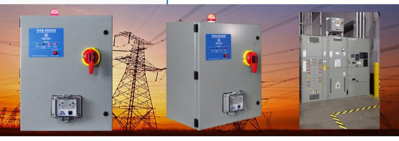
The Tier 800AF Series Arc Flash Relay System reduces arc flash incident energy and boundaries in both Medium-Voltage and Low-Voltage electrical systems. The Tier AF series is an externally installed control cabinet that uses up to four fiber optic sensors to immediately detect light associated with an arc flash event and quickly activate a system disconnect.
